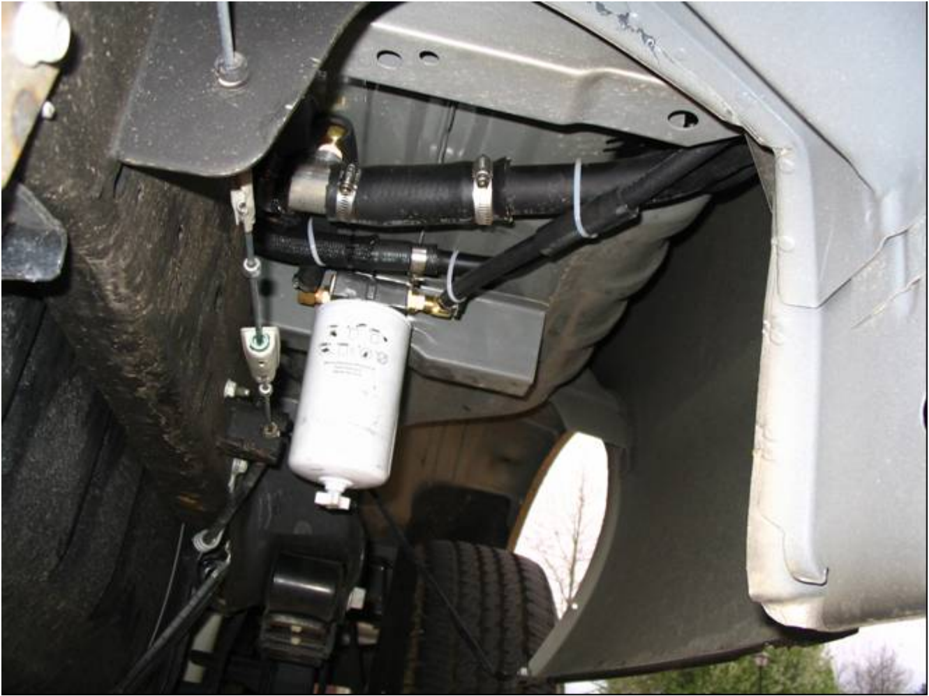
Figure 5. Another pic of the filter and filter housing. You can see the RDS check valve at the top center in the OEM fuel fill hose (note the use of radiator hose to protect the valve and fuel hoses). The 3/8" fuel input line is seen on the right. Despite its open location, I've never seen any physical damage to the fuel filter after over 20K miles of driving, including many miles on gravel roads. Note how the easy accessibility of the filter drain. (Photo by author).
