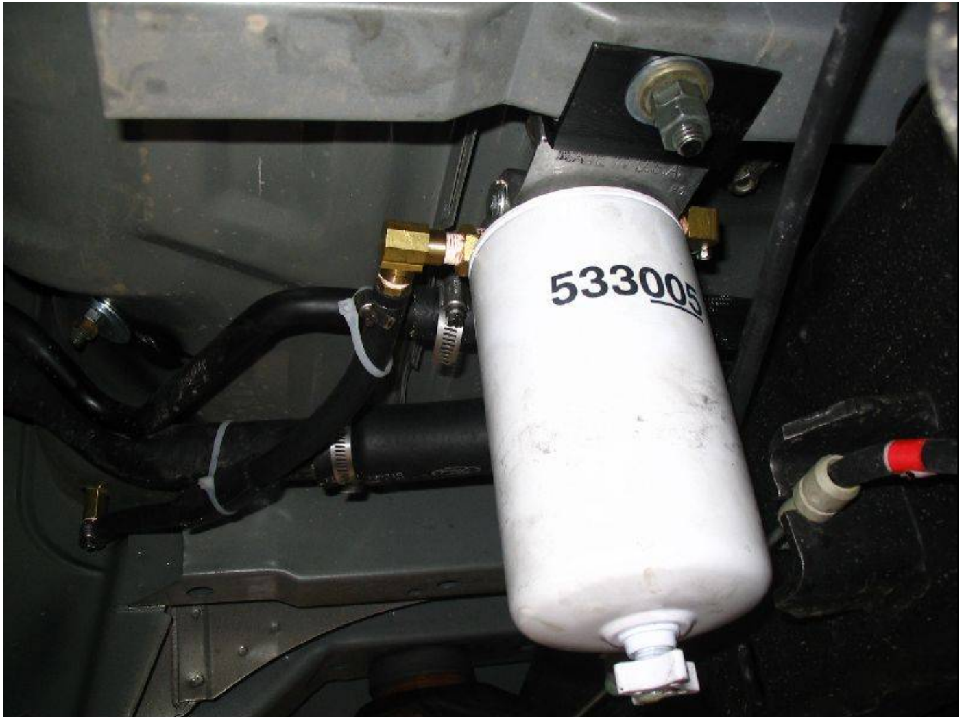
Figure 4. Pic of the Perma Cool 81974 fuel filter mount and 81000 equivalent to the Wix 33005 /NAPA FIL 3005 water separator fuel filter (this filter has since been replaced with a Wix 33405/NAPA 3405 filter). Note the drain on the bottom of the fuel filter; this filter is far easier to drain than the HFCM fuel drain for the '06 PSD. Incoming fuel comes through the hole on the lower left to the 3/8" NPT brass fitting top center; output to the OEM fill hose comes out of the top right 5/16" NPT brass fitting. (Photo by author).
