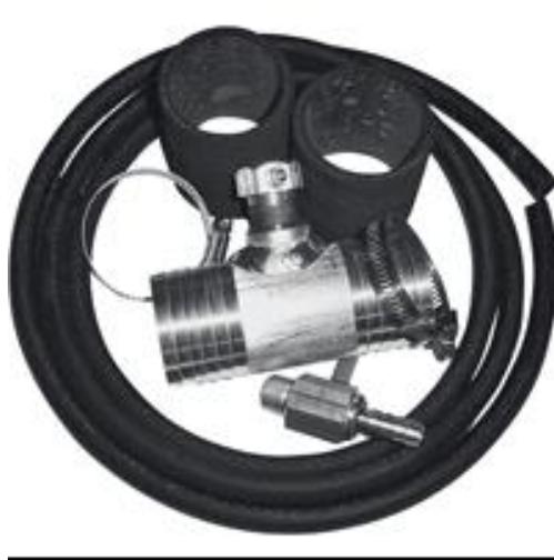
Figure 3. NT/RDS Gravity Feed kit for the Ford PSD truck. The large “tee” in the center of the pic contains the check valve that prevents the aux fuel tank from overflowing the OEM main fuel tank. (Photo courtesy of Northern Tool)
