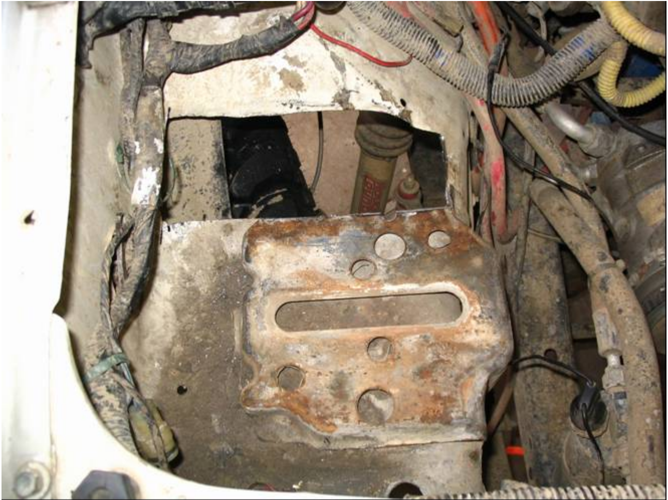
Figure 3. Left fender well area cleared out to make room for dual battery tray. Note the black/muddy fender flare material to the left of the cut out area plus the tire just below it. Cut these areas carefully! The bottom horizontal cut is level with the raised OEM battery tray in the center of the picture. The top black A/C sensor to the right is about \frac{1}{4} " higher than the raised battery tray area and therefore interferes with the dual battery tray. See the text on how I dealt with this.
