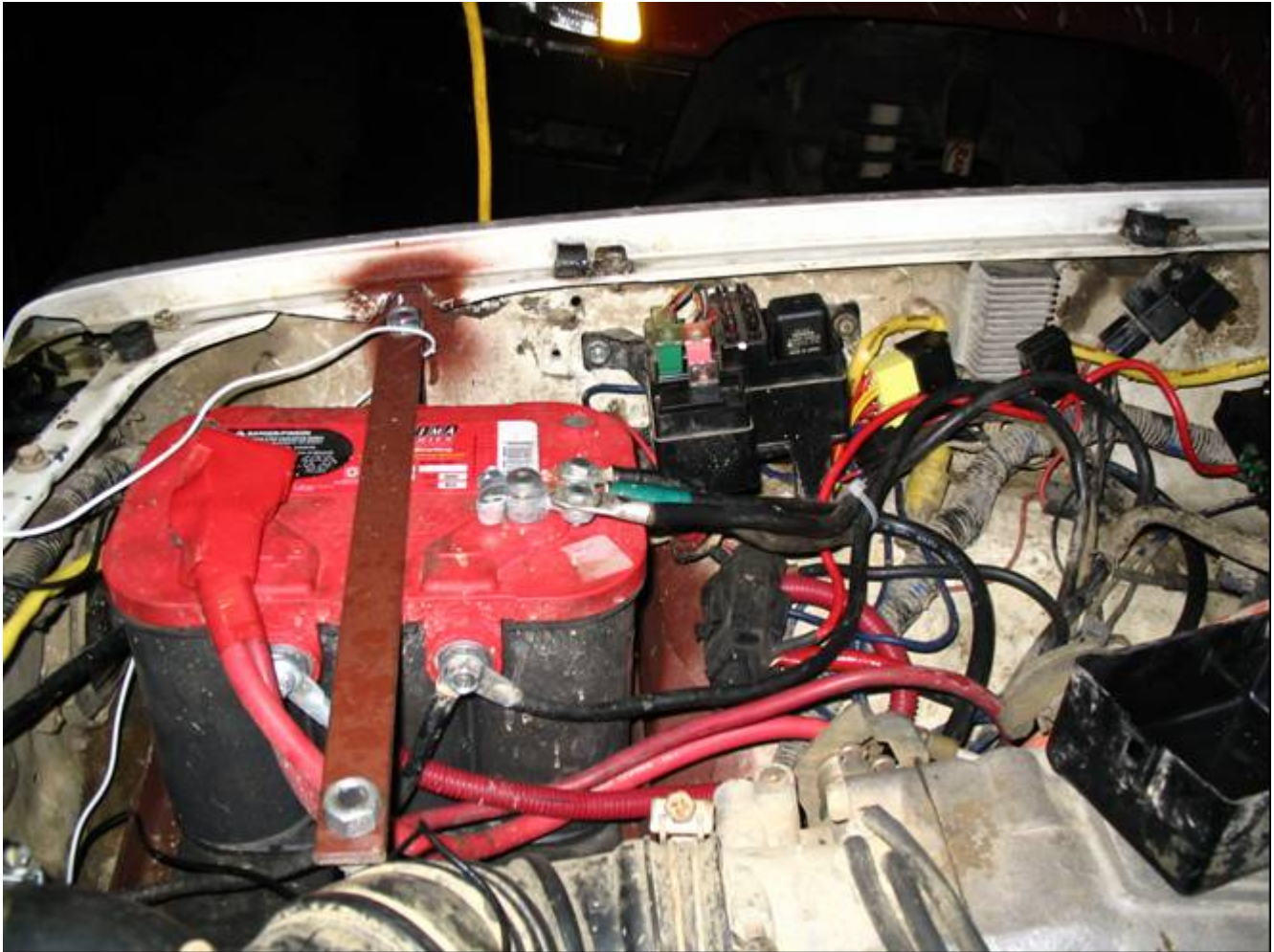
Figure 7. A picture taken for another reason, but the only I have that shows my one Optima battery installed in the dual battery tray. Note the battery hold down bar, the left fender clearance in the upper left and the black 175 amp fuse block for the high power 140 amp alternator just to the right of the battery and below the OEM fuse block. Although it's not clear from this photo, there is room for 2 Optima batteries. Ignore white wire at top: I was in the middle of an aux light install when taking this pic.
