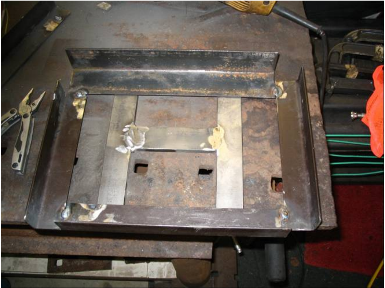
Figure 5. Dual battery tray on top of “H” substructure. Note that the tray has been tack welded and cracks have already formed on the upper right of the tray. The battery tray material is 1 ½” bed frame angle and is hardenable. You must “temper” this material after welding to prevent cracks during service. Regular angle material does not require this tempering. Inside dimensions of the tray is 10” x 14” plus about a ¼” in both directions; just enough to clear two Optima batteries.
